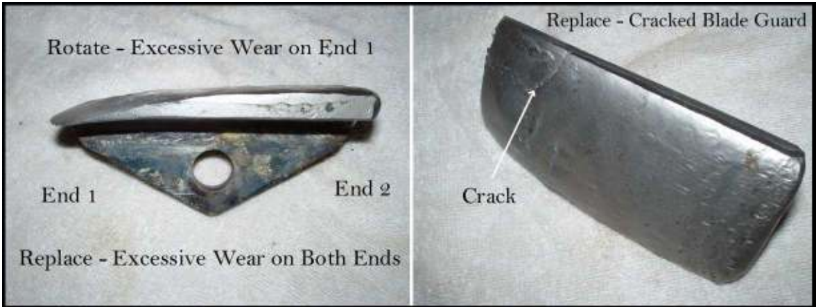
Figure 5 – Excessively Worn or Damaged Blade Guards
