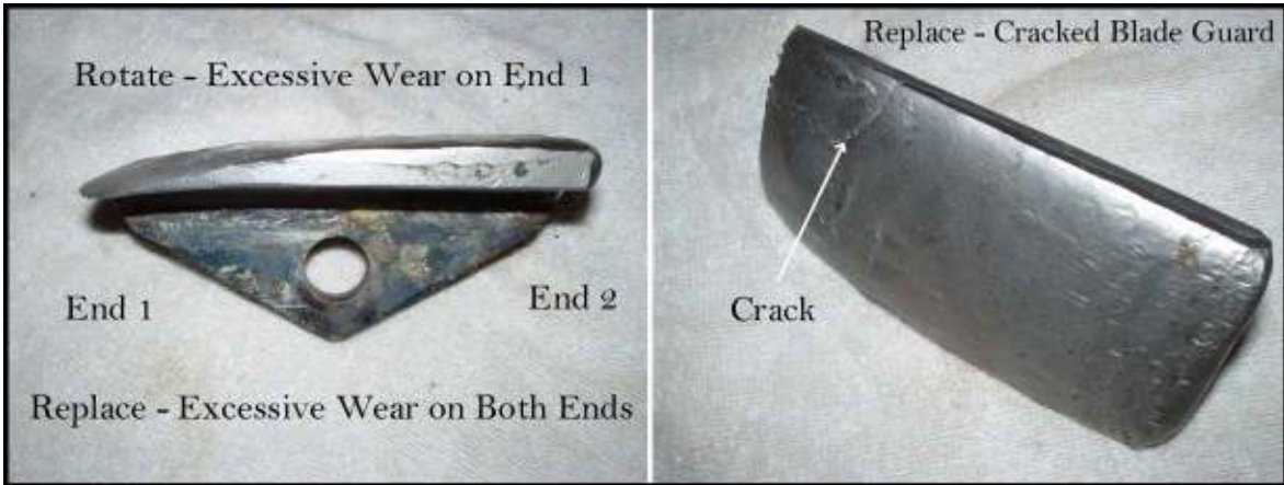
Figure 5 – Excessively Worn or Damaged Blade Guards
